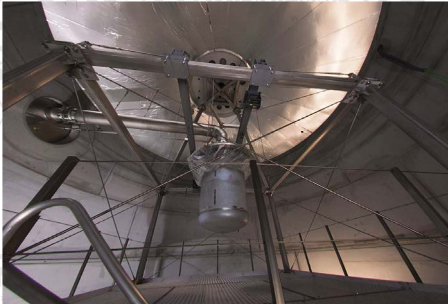
The XENON1T cryostat, under construction in its 10m water tank
